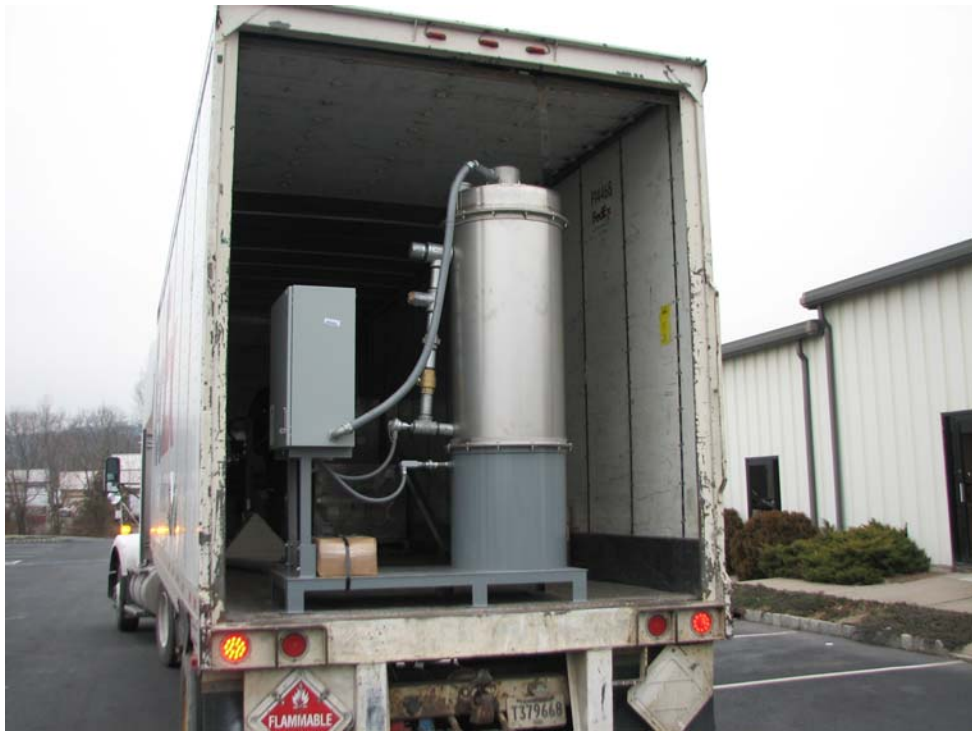
300 SCFM ELECTRIC CATOX SYSTEM
