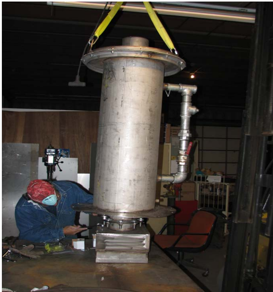
150 SCFM Catox Shell with EZ-Bolt on Type Catalyst Module
