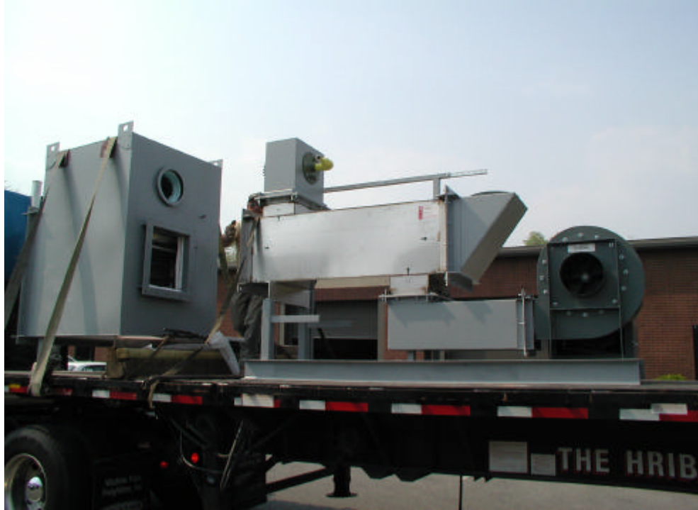
2,000 SCFM Catalytic Oxidizer with Preheat Exchanger
