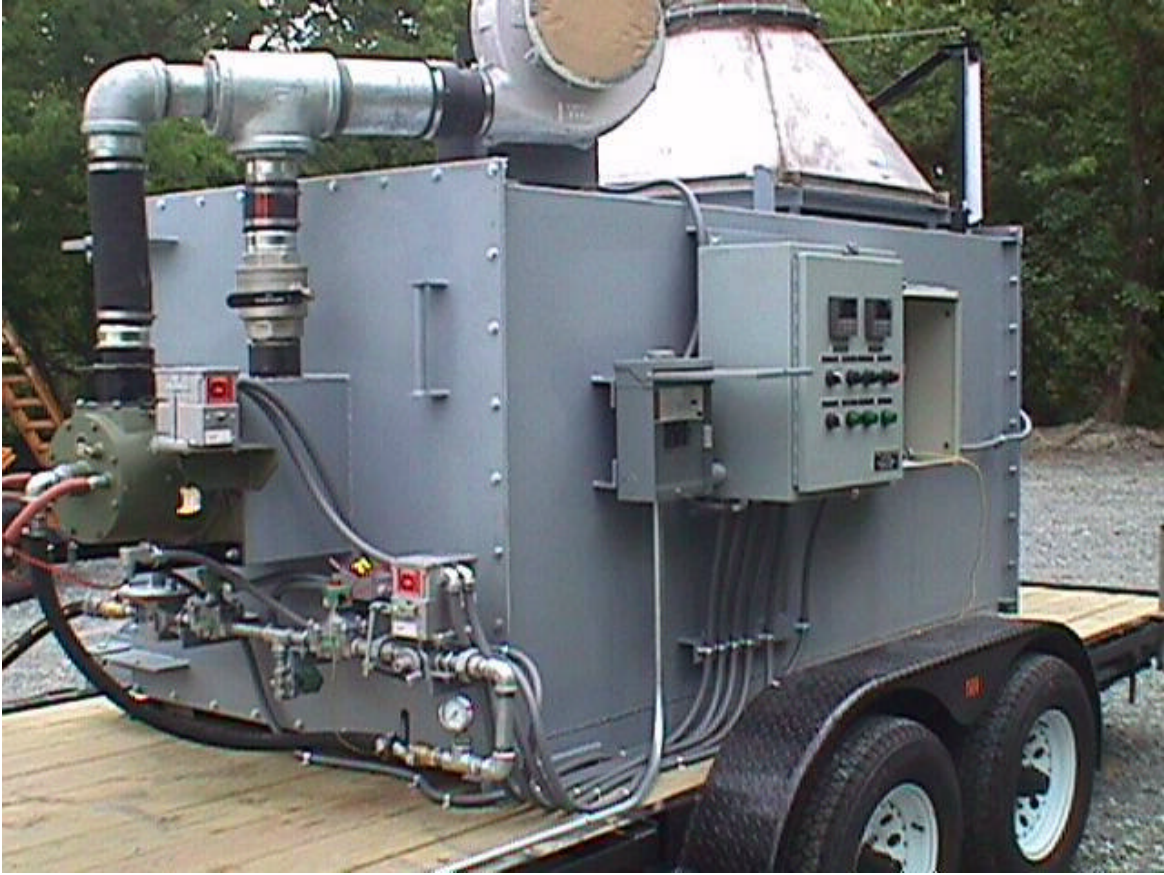
1000 SCFM THERMAL OXIDIZER – TRAILER MOUNTED
