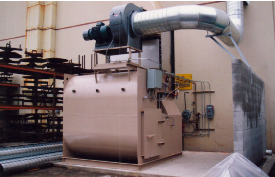
10,000 SCFM Catalytic Oxidizer with Preheat Exchanger (5 Weeks Deliv.)
